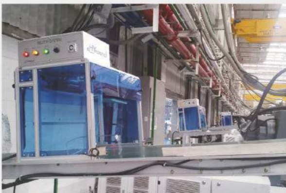
▲ Static electricity removal Conveyor (Light irradiation type)
