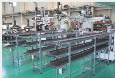
▲ 3 Stage stacking conveyor
