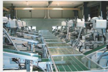
▲ Main and sub conveyor
