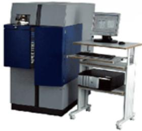
Scanning Electron Microscope (SEM)
