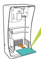
Possible to adjust the height of the container stand (spacer), according to various types of the anti-septic solution containers.
