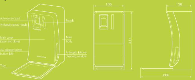
Name and structure Purehygen PH-01/PH-02 (automatic door, air towel KTM series compatible) Material ABS white color Optimal Temperature 5~40°. Humidity 20-80% Weight 1,4kg (except the battery and the empty vessel)
